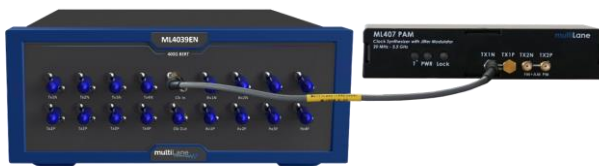
Figure 12: JTOL Test Setup
